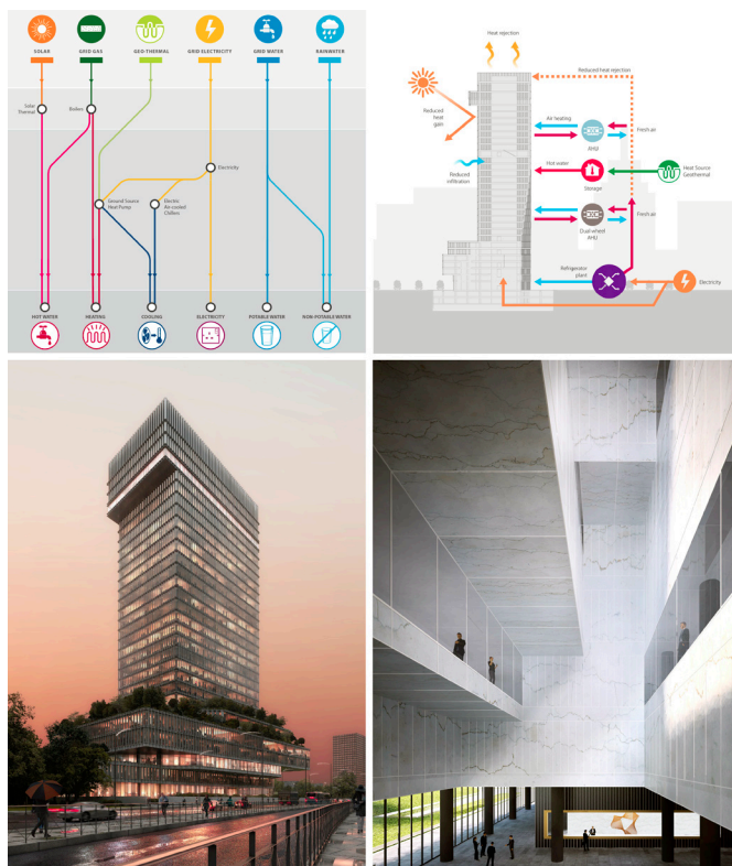
Figure 10: Energy stream and outline HVAC schematic (simulations BuroHappold; north-west and atrium views Mecanoo)
