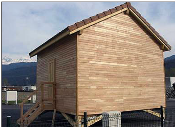
Experimental cell from partner institute CSTB Grenoble used for assessment of heat-air-moisture flows in buildings and constructions
