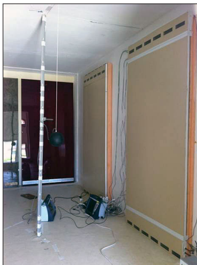
Experimental investigation of innovative ventilated wall element. Left: Facility for assessing airflow using PIV measurements. Right: instrumented wall installed in Passys cell
