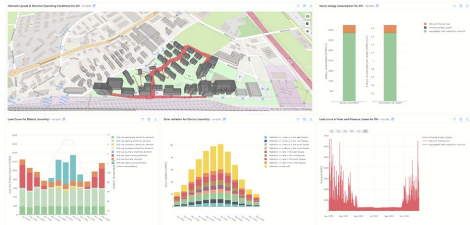
Example analyses on one district from energy demand, solar potential, to district heating network design and operation. Result visualizations on the CEA graphical user interface
