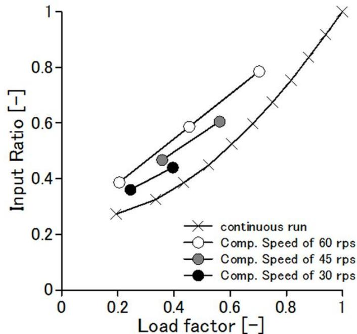
**Figure 3.** The relationship between load factor and input ratio
