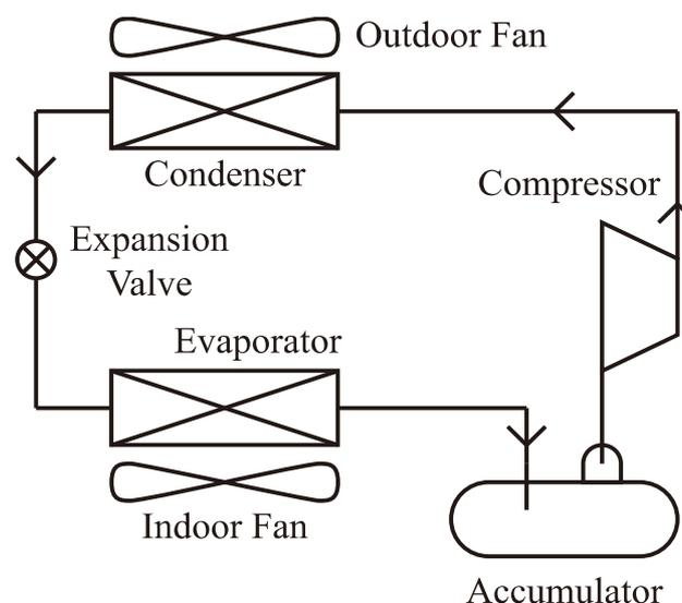
*Figure 1. Schematic view of heat pump*
