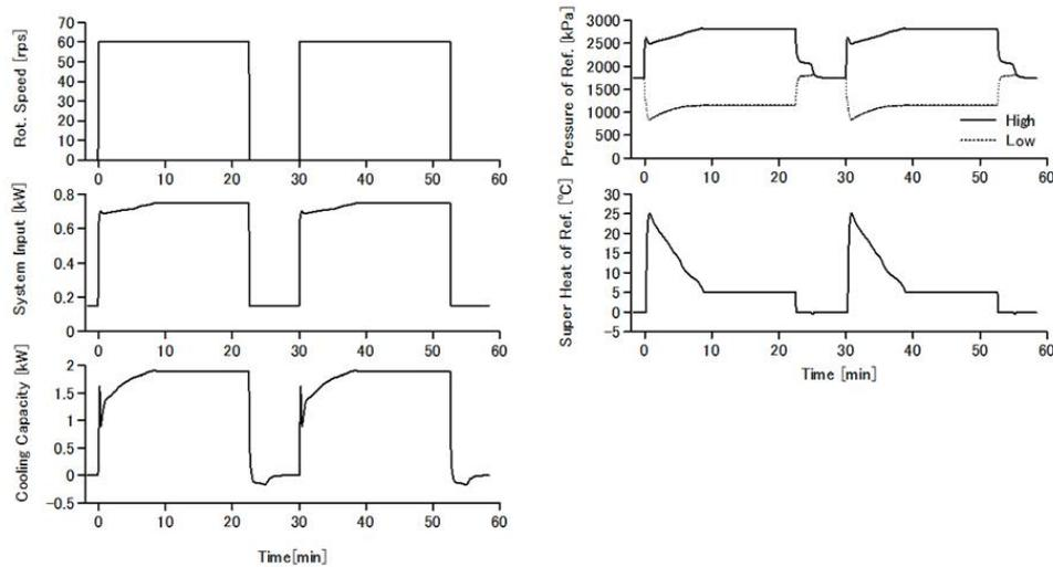
**Figure 2.** Results of numerical simulation for intermittent operation
