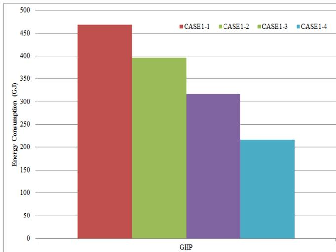
**Figure 4.** Comparison of the energy consumption for a single geothermal system.
