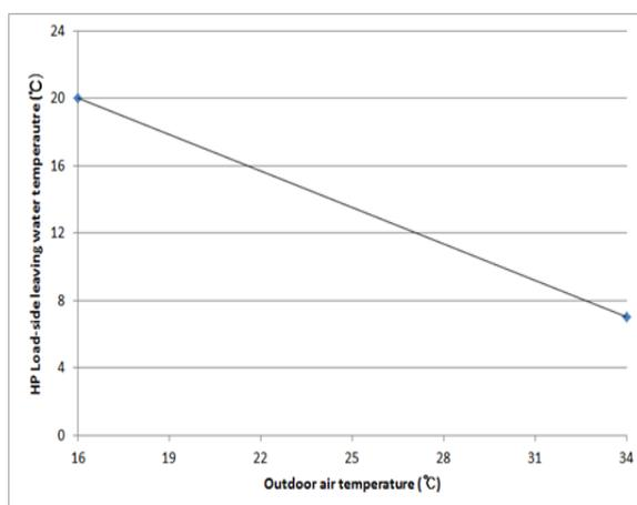
**Figure 2. Outdoor reset control curve**
