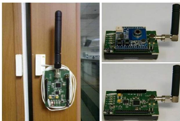
*Figure 1. A sensor nodes with various sensing modules*
