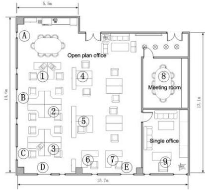
**Figure 1.** Office plan and testing points
