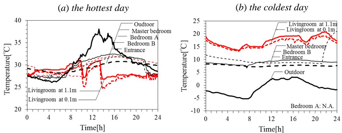
Figure 2. Temperature fluctuations on the hottest day(a) and the coldest day(b)of the measurement period
