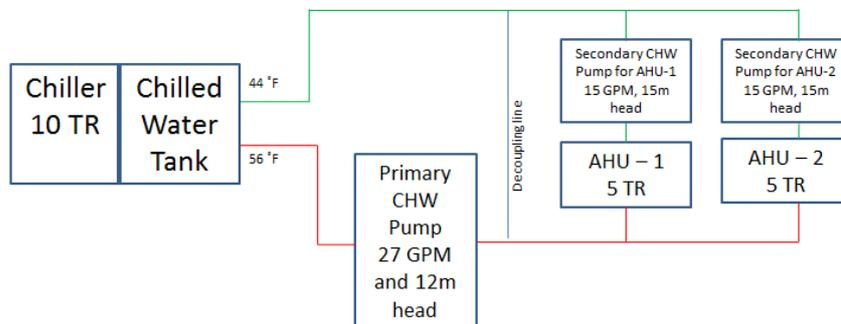
**Figure 3** Schematic of water side system
