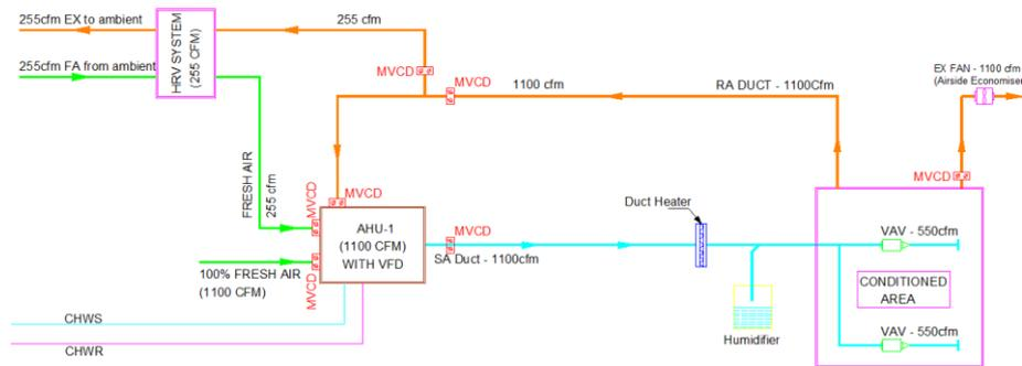
**Figure 2** Schematic of air side system
