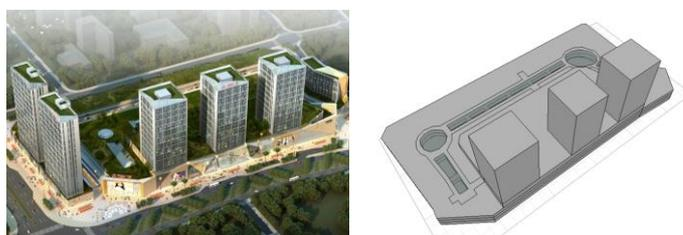
**Figure 5.** project which fails to model all significant neighboring obstructions
